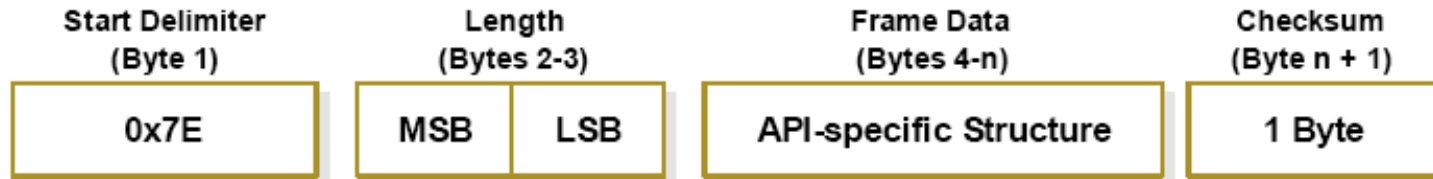
Figure 4-01. UART Data Frame Structure:
