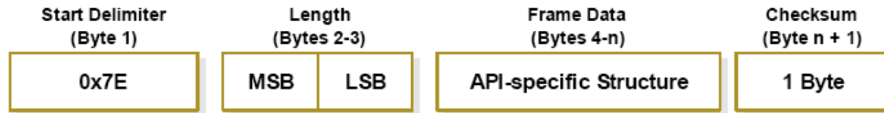
Figure 4-01. UART Data Frame Structure:
