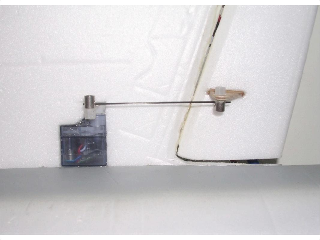
Motor + Potentiometer + Microcontroller
